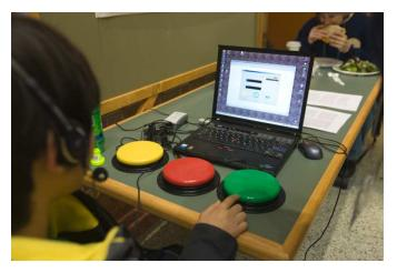
Fig. 1. Hardware setup for the *Speech Recognition Game*. Red, green and yellow external buttons were used to accept all non-speech user inputs. A green bar, displayed on the computer monitor, rose with each recognized word, to peak at ten correct recognitions.
